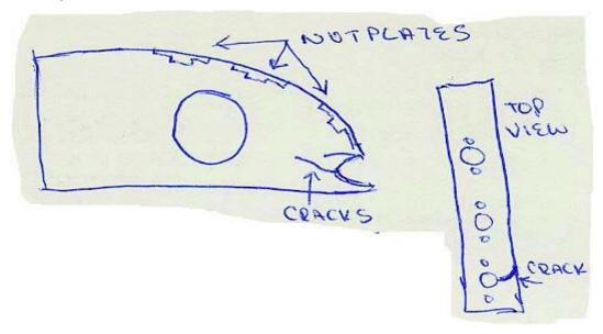
(This technician also includes another such report of a cracked attach point for the flap actuating rod on a Beech 55 having 4,552.7 hours. Of these six above referenced Beech aircraft, the time ranged from 3,144.9—to 5,255.1 hours yielding 2,110.2 hours difference. This is awfully good anecdotal evidence arguing for close attention to these actuation attach points after a couple thousand hours.)
