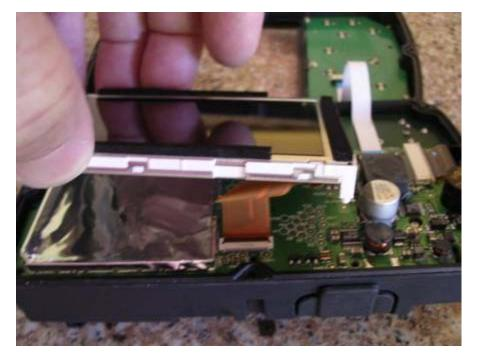
I left the copper colored ribbon in place, but you must remove the red & black "power" wire at the side. To remove this you must hold the base (connected to the board) while pulling the wire plug straight up with tweezers. Be careful or you will have to solder this part on also!
