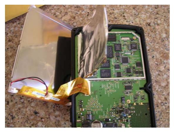
With the screen flopped over you can peel back the foil shielding to get access to the two screws underneath. There are 2 screws under the foil, and 2 screws visible on the board. Remove all 4 screws.
