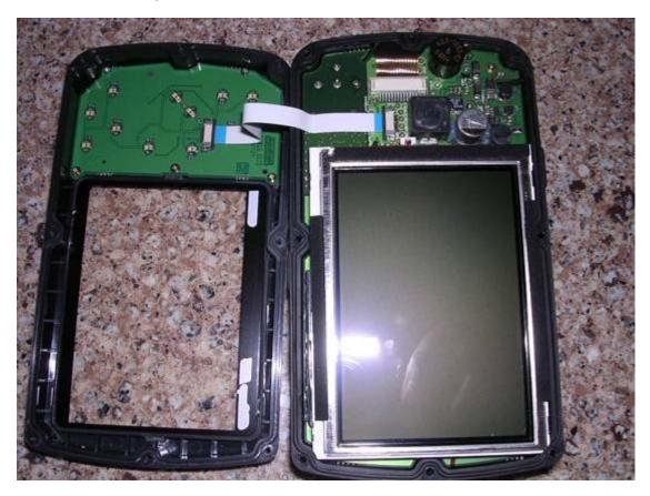
Remove the white ribbon cable that goes top both halves by gently sliding it out of the slot on the "screen" half.
