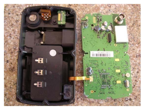
Here's the other side with our round coin battery. The stock battery is made in Germany and rated at  $3VDC \sim 7mm$  diameter. It is soldered to the board with 2 tabs. The tabs are spot welded to the battery. Use a Volt Ohm meter to verify the +/- direction and write it down.
