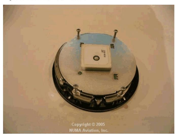
8. With the circuit board exposed, remove the three screws circled.
