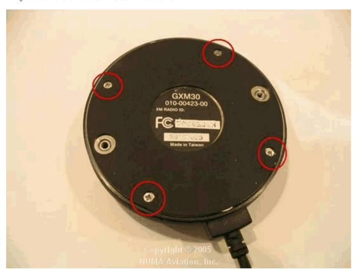
3. Flip the antenna back over and CAREFULLY lift the top cover a little.
