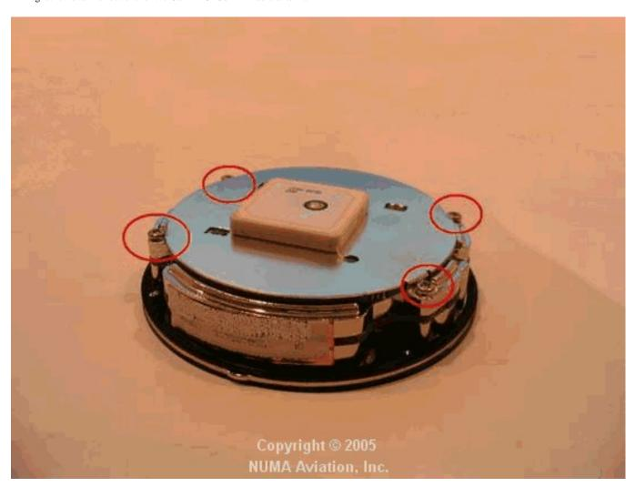
7. Once the screws have been backed out, remove the top cover.
