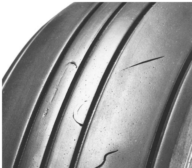
Cuts Penetration by a foreign object. See Section 4, Inspection, Storage and Shipping; Inspecting Mounted Tires; Tread Cuts.
