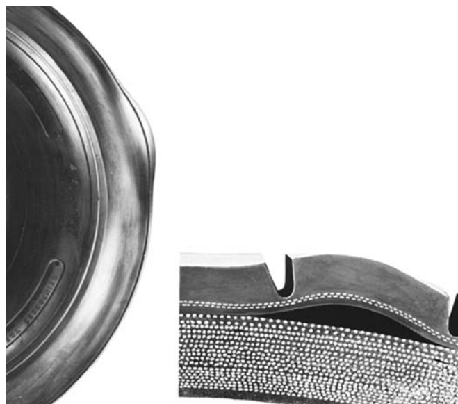
Tread Separation A separation or void between components in the tread area due to loss of adhesion, usually caused by excessive loads or flex heating from underinflation. Remove immediately.
