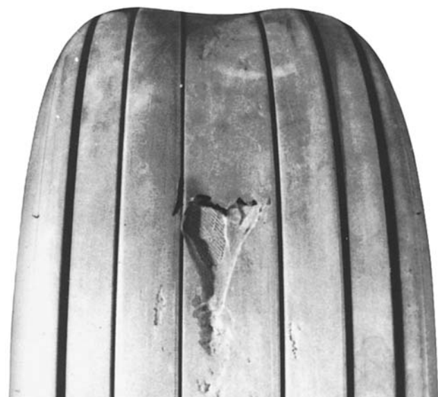
Tread Chunking A condition in the wearing portion of tread usually due to rough or unimproved runways. Remove if fabric is visible.
