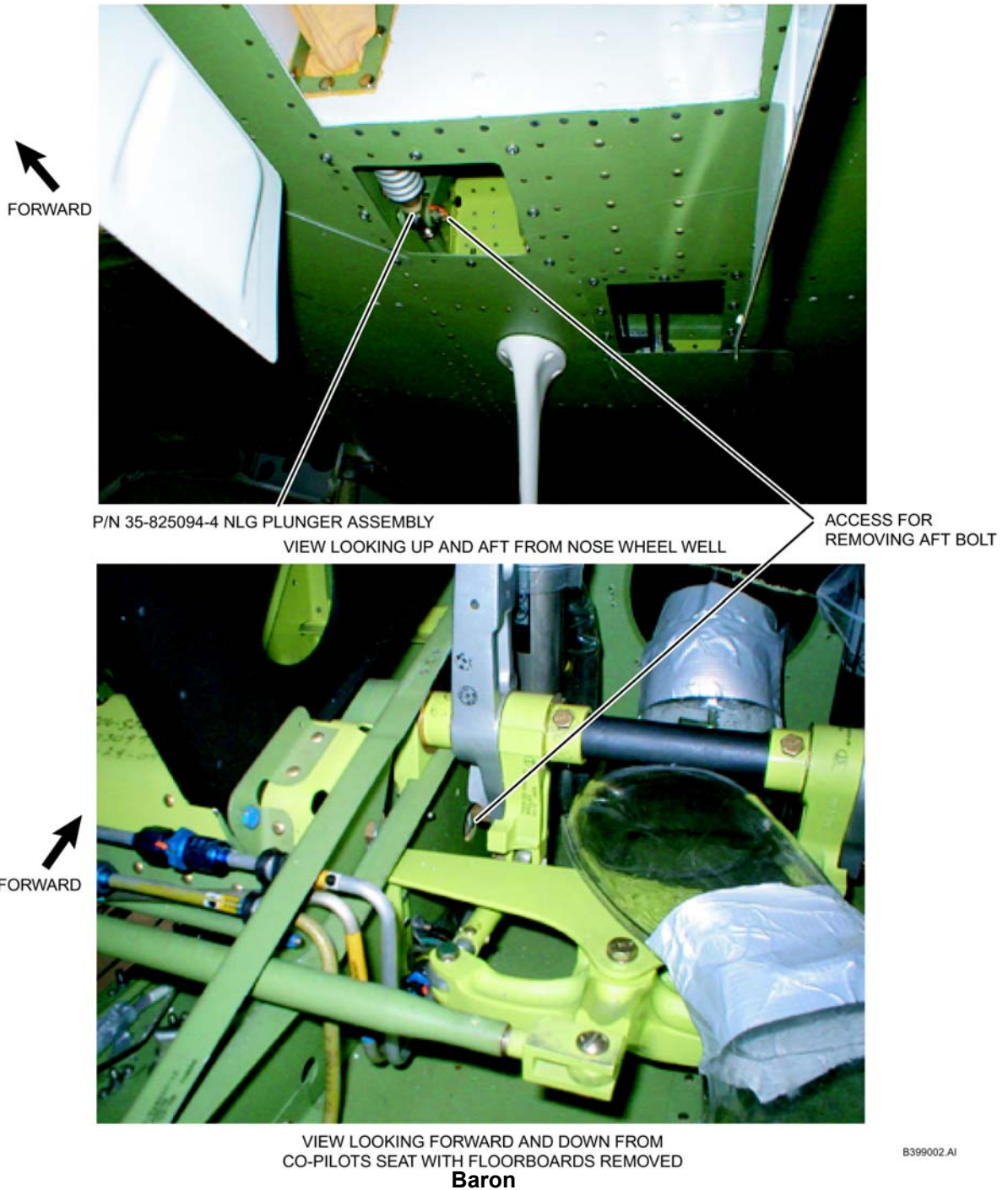
Access Points for Removal of Retract Rod Assembly in Nose Wheel Well
