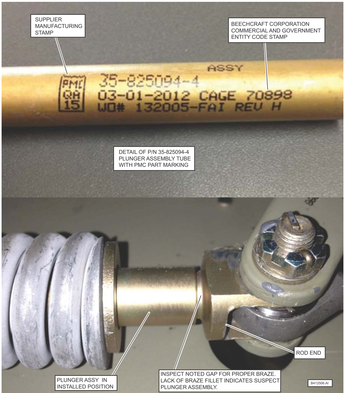
PMC P/N 35-825094-4 NLG Plunger Assembly Braze Inspection
