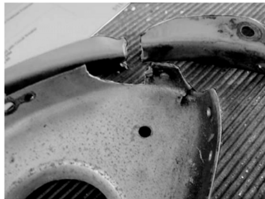
EXAMPLE OF TORN FLANGE IN P/N 35-165050-84 WITH NUTPLATE MISSING
