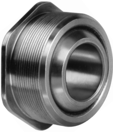
This aircraft flanged spherical bearing uses a threaded O.D. to provide a retention feature. The threaded O.D. also allows for ease of replacement in the application.
