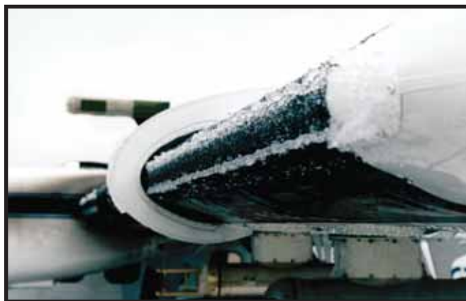
Clear ice formation on wing leading edge
