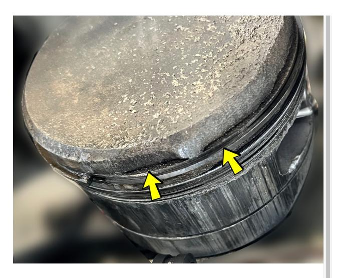
"With the cylinder removed, the full extent of piston damage was obvious," Roy noted. "The engine had 1,540 hours SMOH, but ironically had a top overhaul only 100 hours ago due to the ECi cylinder AD. At this point it's obvious that the #1 cylinder needs to be addressed, and I'm thinking it should probably be scrapped and replaced due to the way-over-red-line CHT and consequent metallurgical trauma. The piston is obviously trashed, too."
