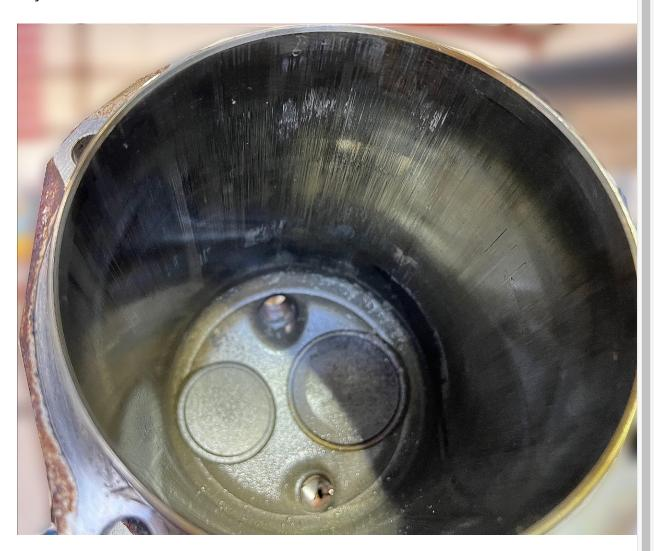
"A borescope inspection of right engine cylinder #1 revealed scoring of the cylinder walls and some corner melting of the piston," Roy continued. "The shop asked for permission to pull the cylinder, which I approved since it seemed obvious that this needed to be done."
