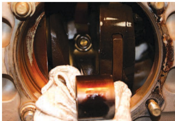
Figure 2.- Crankcase internals heavily painted with varnish
