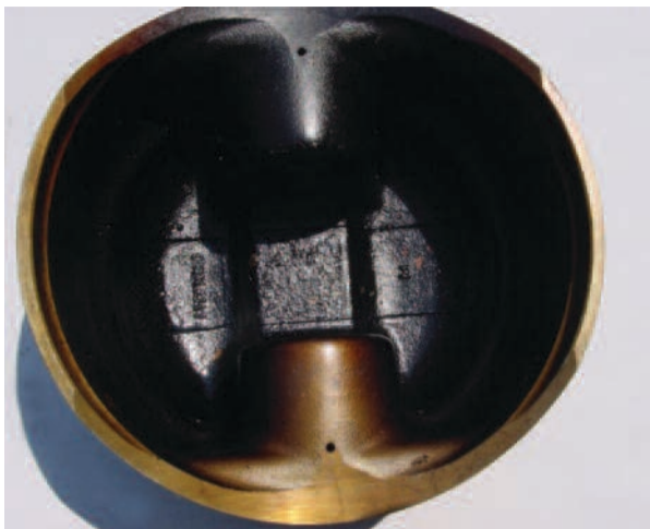
Figure 3. Underside of a piston with a carbon film deposit
