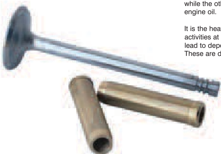
Figure 1: Valve and valve guides. Courtesy CB Performance
