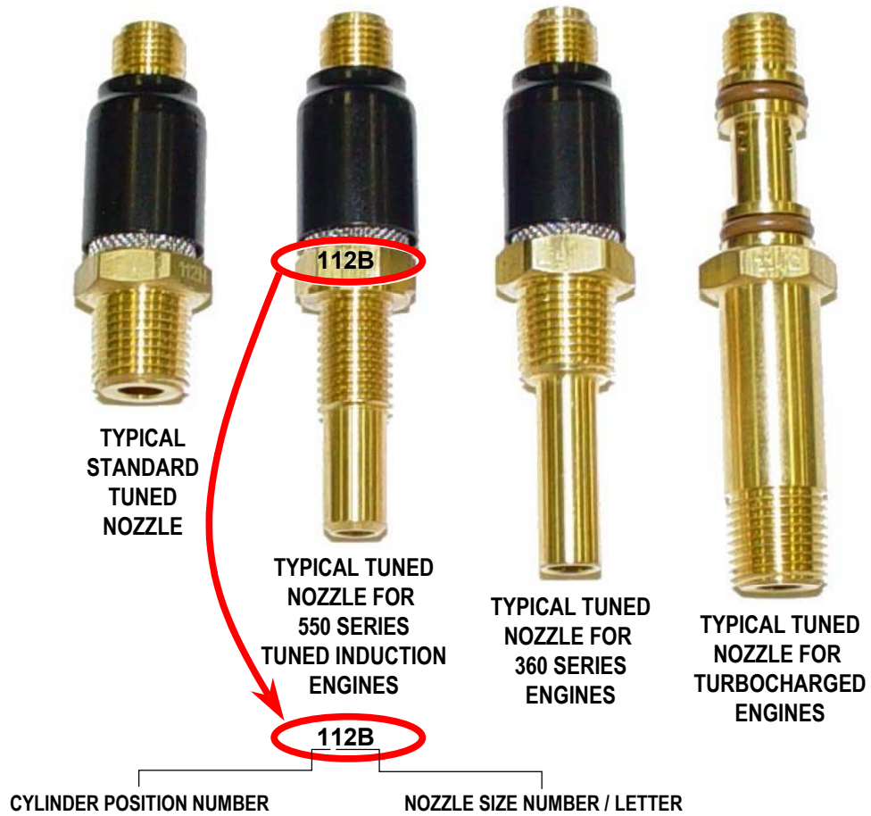
Figure 3. Nozzle Position Marking
