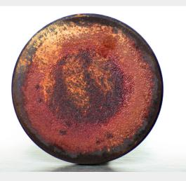
Don't be alarmed by the bright color, or deposits around the edges. The symmetrical pattern shows this valve is just fine.
