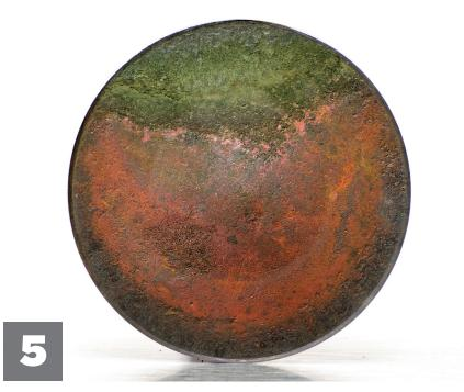
Green crescent progresses toward center with valve cracking and failure a serious danger.
