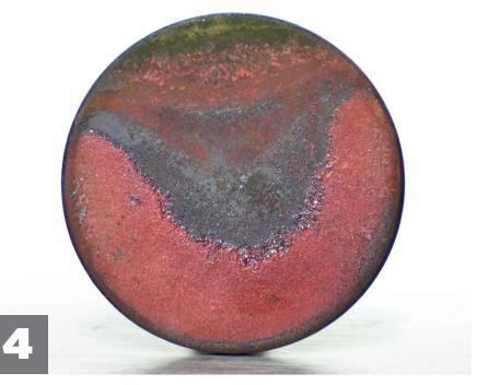
**GREEN MEANS STOP.** The green area at the top shows this **valve should be replaced immediately.** (Note how the uneven burn patterns match the heat distribution chart.)
