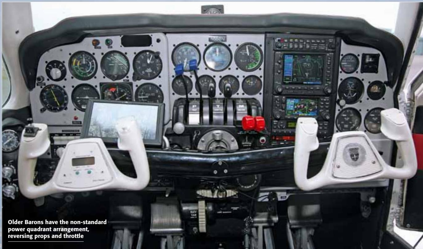
**Older Barons have the non-standard power quadrant arrangement, reversing props and throttle**
