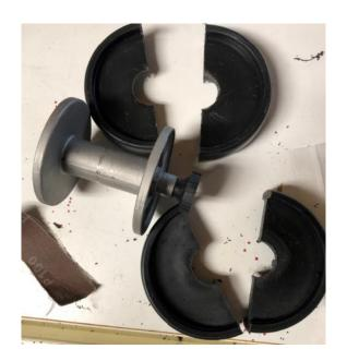
Assemble on the spindle with some tape to hold everything together while you drill through the assembly. I then cut some spacers to slide over the bolts to keep the wheels rigid – you can see I haven't added the last one in this picture to go over the threaded portion. The bolts I think are Grade 5 3-1/2" (everything else is M6).
