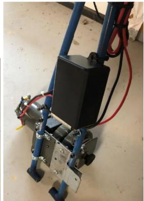
Mounting hardware is large tie-wraps and a hose clamp. And here is the finished project! I may strip it down and paint it, and maybe add some handlebar grips to it just for fun:
