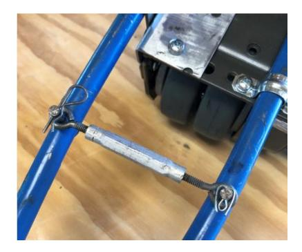
One side is permanently installed with a cotter-pin, and the other has a removable pin. Simply remove that side of the turnbuckle, and attach to the nosewheel pins. Put it back on and turn it to desired tension – now it won't pop off while turning the nose!
