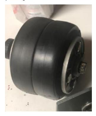
Now, as the other article mentions, now the diameter of the wheels is larger than that of the spindle with cable, the frame needs to be offset to accommodate, and the axle hole will need to come down – this necessitated cutting the frame. Not having access to a welder, I elected to use a metal bracket. I may take it all to have welded now that I know it works. I just cut the frame with a dremel, and added about ½" worth of spacers to clear the wheels and the bracket to bring the axle hole down:
