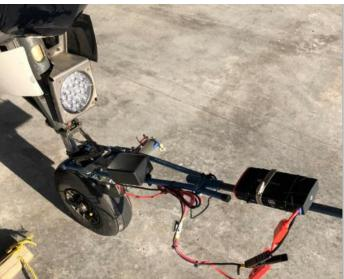
There you have it, another take on the CSOBeech towbar, for less than \$100, and no welding required. I can tow it out of the hangar, put it back on the charger, then use it to get back inside! If the battery dies, I can still use it as a conventional towbar. The middle pin still comes out so it can be broken down for travel.
