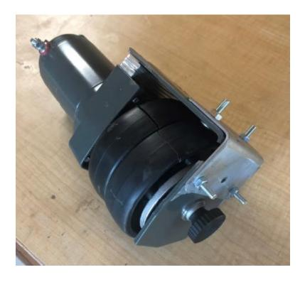
Now, rather than using aluminum U-channel to mount the bar, I diverged a little bit here because I wanted to solve for two problems: 1) being able to hold tension against the nose tire, while still allowing it to move back and forth for mounting ease and 2) being able to hold clamping force against the nose gear pins also while being able to open and close the "jaws" for mounting.
