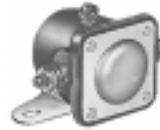
No. 2430 Phenolic Housing Bracket mounting holes 9/32" x 1/2", 2 13/64" on centers.
