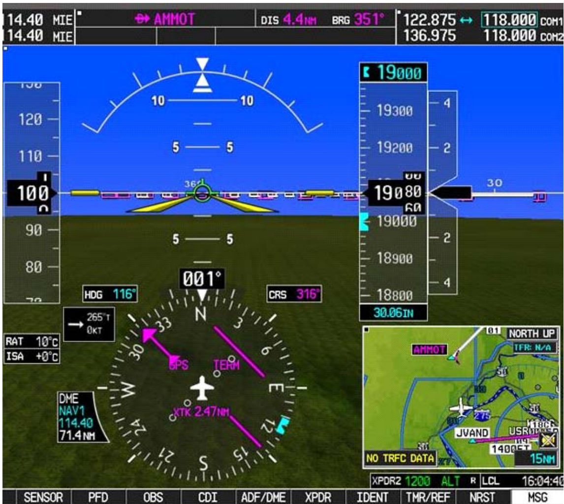
Figure 1. Garmin Integrated Flight Deck System PFD Display While on Second DF Leg
