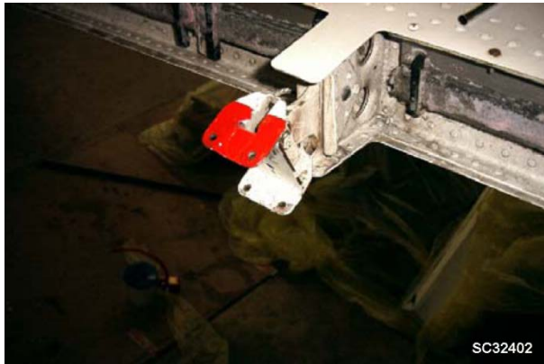
Figure 2 – Witness Mark Painted on Aileron Hinge Bracket (Aileron Removed)
