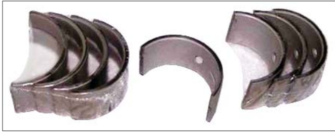
Fig5: Main bearings are semicircular shells held in place by through-bolt torque.
