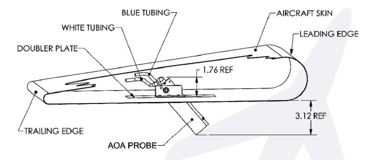
The AOA probe must be mounted solidly to the aircraft, in clean air flow (undisturbed air), a minimum of 2 feet outside the prop arc, typically mounted 6" back from leading edge, 6"up from trailing edge, at any attitude, slip or skid NOTHING disrupting the direct air into the AOA probe.
