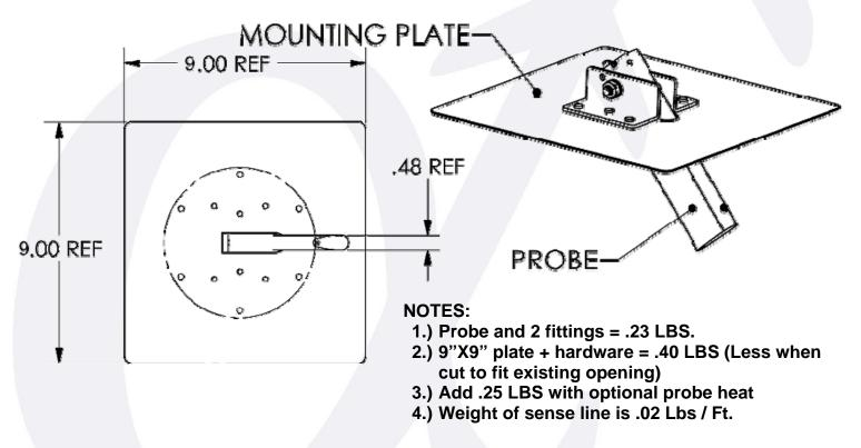
For most aircraft, the AOA probe mounting plate WILL be cut to the shape of an existing inspection opening as outlined in this manual. After the mounting plate and probe are attached to the aircraft, it also may become necessary to remove material on the mounting plate to allow the AOA probe to be adjustable past the 50 degree angle to allow for full scale electronic calibration (if additional angle increase required).
