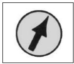
The course selector knob is used to adjust the autopilot course selector arrow to the desired course. Selection of the autopilot course automatically sets the internal VOR resolver to the identical VOR radial. Readout of VOR left-right information is made by observing the center segment of the course arrow
