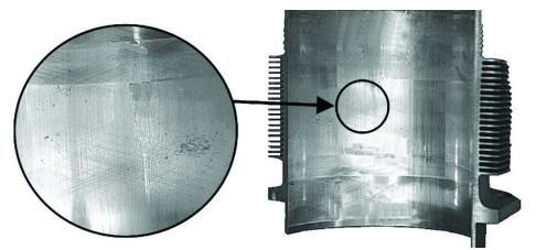
Figure 4. Typical Cylinder Bore at TBO
