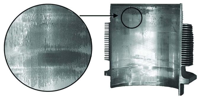
Figure 2. Heavy Corrosion Formation, Surface Pitting
