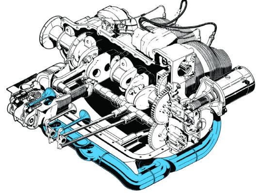
assembly. Air from the manifold is carried into the intake ports, mixed with fuel from the injector nozzles, where it enters the cylinder as a combustible mixture when the intake valve opens.
