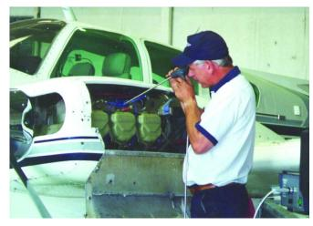
Inspect each cylinder for signatures of normal wear (Figure 4). Cylinder walls which appear to have minimal, or no hone pattern are acceptable if the cylinder has acceptable differential compression readings and the engine has acceptable oil consumption.
