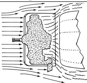
Most of the early four cylinder, horizontally opposed engines were velocity cooled like their radial cousins. However as these engines increased in size, they too had to be pressure cooled. As the aircraft industry grew, the state of the art improved and engine cowlings became streamlined as illustrated in Figure 4. Consequently the space inside the cowling decreased. The proper cooling of engines in such aircraft now became an exacting science.
