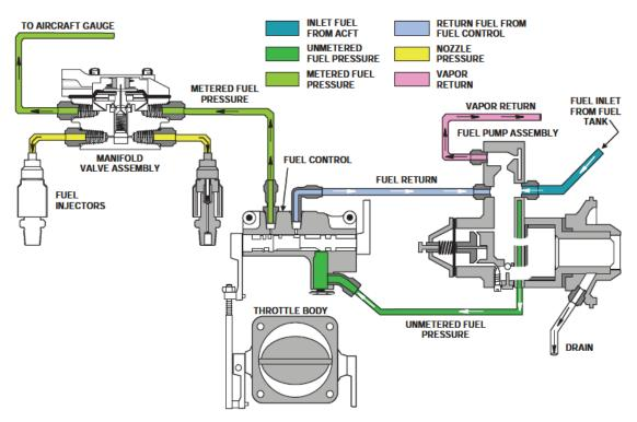
**Typical Naturally Aspirated Fuel System Schematic**
