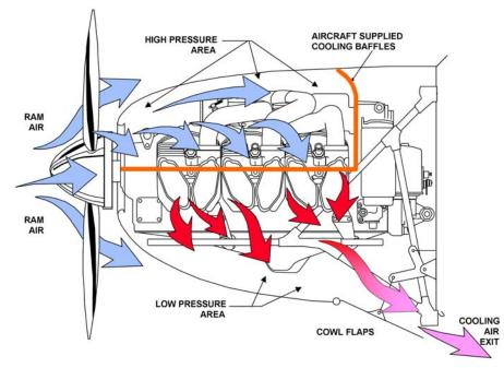
Notice how air entering the cowling opening in the front is forced around the cylinders by means of baffles and moves into the lower cowling where it passes overboard through the cowl flap openings. Cooling air also enters the accessory section via strategically located vents
