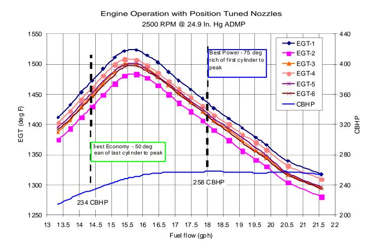
Figure 3. Engine Performance After Optimization
