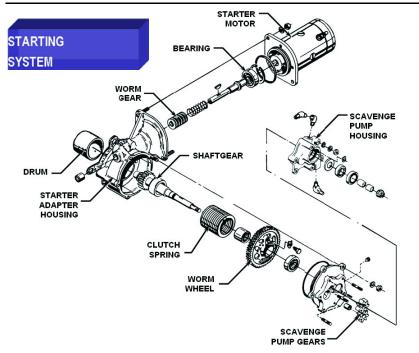
Permold Engine Starter Adapter with Scavenge Pump
