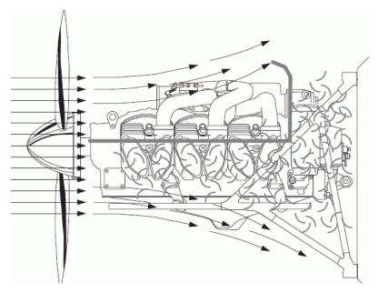
Figure 5 illustrates proper airflow around the engine's cylinders and as stated earlier this is possible only when the upper cowling is pressurized. Now look at the same illustration in Figure 7 only with the cowling removed. Notice that air is flowing over and around the engine but not around the cylinders where it is needed most. While this is an illustration, it is no exaggeration. Running a pressure cooled engine without its cowling simply will not provide adequate cooling.
