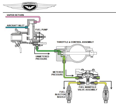
The process will be different for Continental engines equipped with a mixture control on the fuel pump. This type of fuel injection system is employed on the 240 and 360 series engines and the IO-550-G, N, P & R engine models. With this type of system you will need to run the boost pump for 20 seconds and then open the mixture control until a metered fuel flow indication is present on the instrument gauge.
