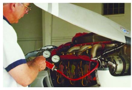
Cylinder walls, ring surfaces, and valve seats are subjected to wear throughout the life of an engine. At regular maintenance or when condition inspections are indicated, differential pressure checks should be performed and recorded for trend monitoring.
