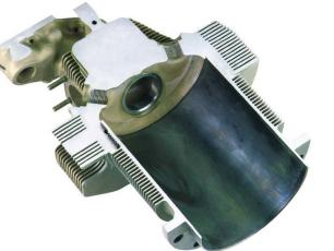
The main problem with inactivity is the lack of a protective coating on engine parts. The longer the engine sits inactive, the lubricating engine oil "falls" away from the steel parts, exposing them to the atmosphere. Of course we all know that steel rusts in that atmosphere here on planet earth. So, as long as we fly here on this planet, we need to be aware of the problem of rust and corrosion. Steel rusts and aluminum corrodes.
