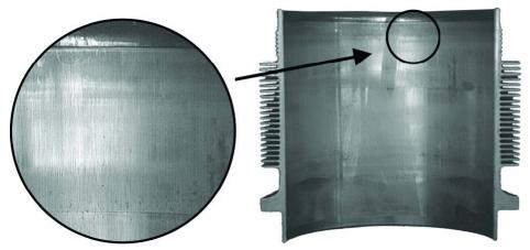
Figure 5. Heavily Worn Cylinder Bore
