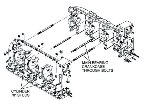
main bearing saddles that will house precision tri-metallic crankshaft main bearing inserts. Guides are bored through lateral bosses at the main oil transfer galleries to support the hydraulic valve lifters.
