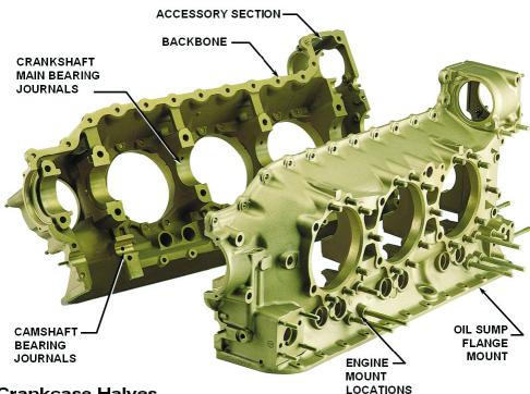
crankshaft, camshaft, and main bearings. It also provides external surfaces for mounting the cylinders, as well as all other external engine mounted components, such as the oil and fuel pumps, induction and exhaust systems, magnetos, starter motor and starter adapter (on six cylinder models), alternator, and oil cooler. Aircraft supplied accessories such as a propeller governor, vacuum pumps, and standby alternators can also be mounted to the engine.
