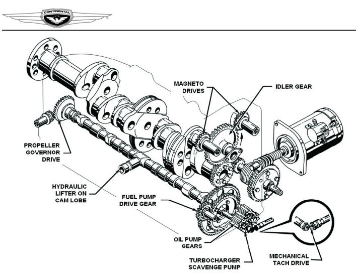
**Typical Six Cylinder Gear Train**
