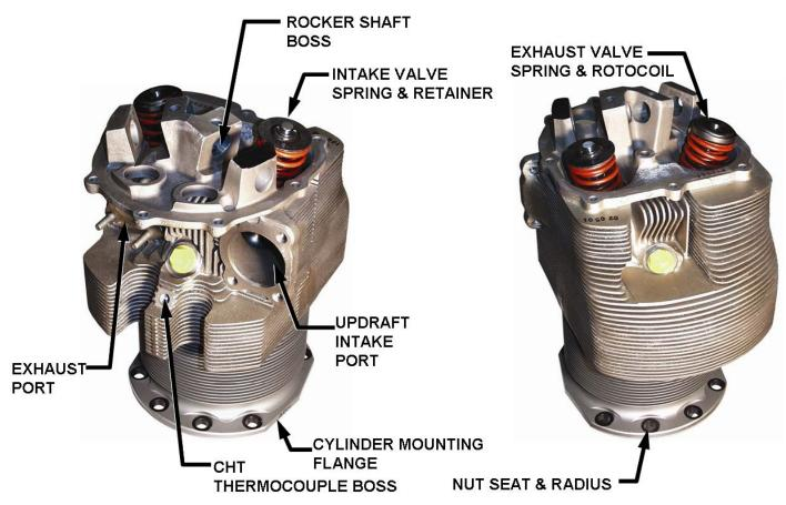
Cylinder assemblies and their related components are subjected to a severe operating environment. Although many operational factors can contribute to the deterioration of a cylinder's durability, the loads resulting from combustion pressure and operating temperatures are the largest. The number of engine starts, or thermal cycles is also a contributing factor. Corrosion of the cylinder head and barrel can destroy the durability of a cylinder rapidly.
