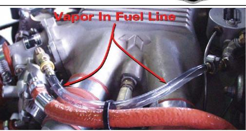
Figure 3. Heat Soaked Vapor in Clear Line
