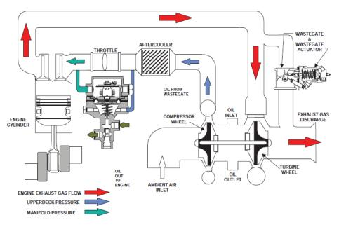
(deck pressure) is regulated by controlling the flow of exhaust gas through the turbocharger turbine. This is accomplished with a hydraulically controlled exhaust by-pass valve (wastegate) in the exhaust system prior to the inlet of the turbine housing. The wastegate valve is spring loaded to the open position and closed by pressurized oil from the engine.
