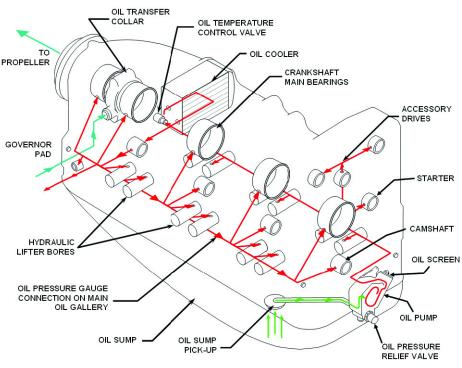
Sandcast Engine Lubrication Schematic
