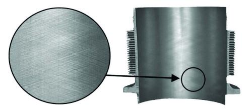
Figure 3. New Steel Cylinder Bore
