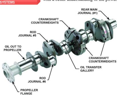
The Power Train section of the engine consists of the engine crankshaft, connecting rods, camshaft and accessory gear drives. We will discuss each of these in order to provide you with a better understanding of the powerplant in front of your aircraft.
