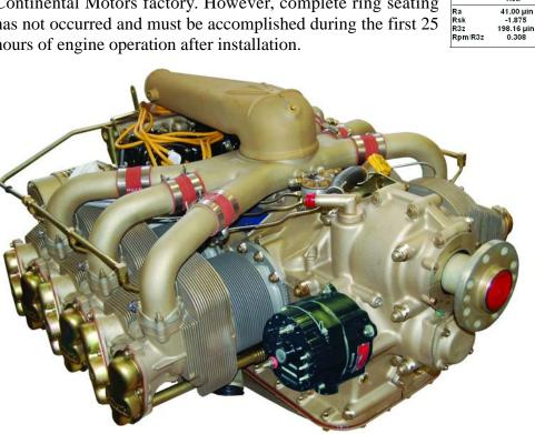
Piston ring seating is paramount to proper engine break-in. Understanding the factors involved in the break-in process will aid in correctly operating the engine during this critical period. Piston ring seating means the rings and the cylinder wall must wear-in together to provide an effective seal for the combustion chamber and to keep combustion gas blow-by and oil consumption to a minimum.
