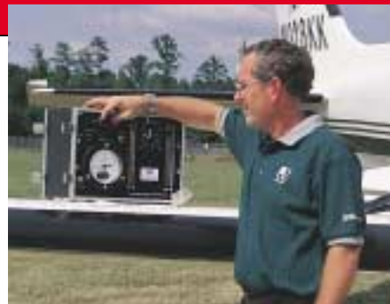
Paul Cramer of Kelly Aerospace is using a Porta Test unit manufactured by Aero Test, Inc. to set fuel pressures on a Cessna 340.
