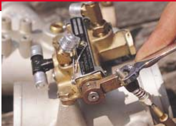
This is a typical 470 and 520 mixture style adjustment. It requires a 3/8 wrench with a clockwise rotation to enrich the mixture.
