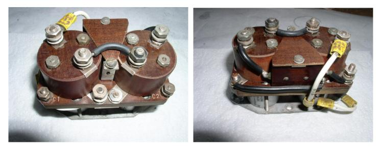
3. This is how the relay looks once removed and on the workbench. The left photo above shows the relay positioned as installed in the airplane, looking from the back seat perspective. The right photo shows the forward side of the relay. Compare these views with the photos at the opening paragraph to better see other connections, the solenoids and related wiring. Terminals are marked with letters and/or numbers (C1, C2, etc.) to denote external connections to other system components.
