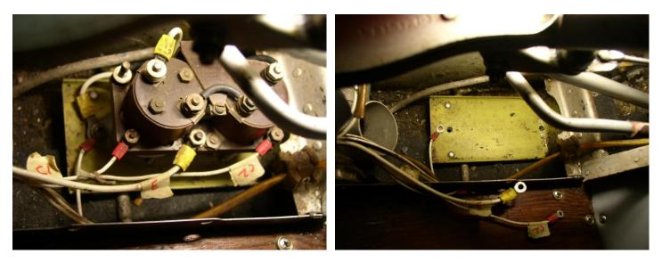
2. Begin relay removal by marking all the wiring connections, as shown above left. The motor wiring has already been removed in this photo. The wires can be disconnected either with the relay mounted or after removing the two relay mounting screws and lifting the relay from its mounting plate (as shown above right.) If wires are disconnected in place, be very careful not to drop the small terminal nuts and washers down into the underfloor areas since access is quite limited.
