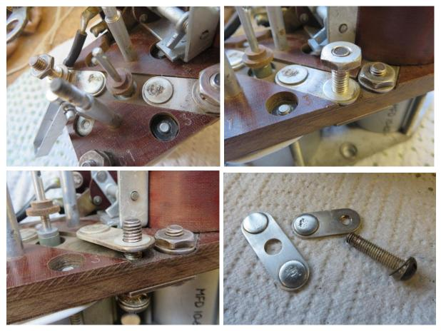
4. A good ground connection is critical to proper braking function. The photo shows the relay tray ground screw location, which should be cleaned of paint for the best conductivity.
