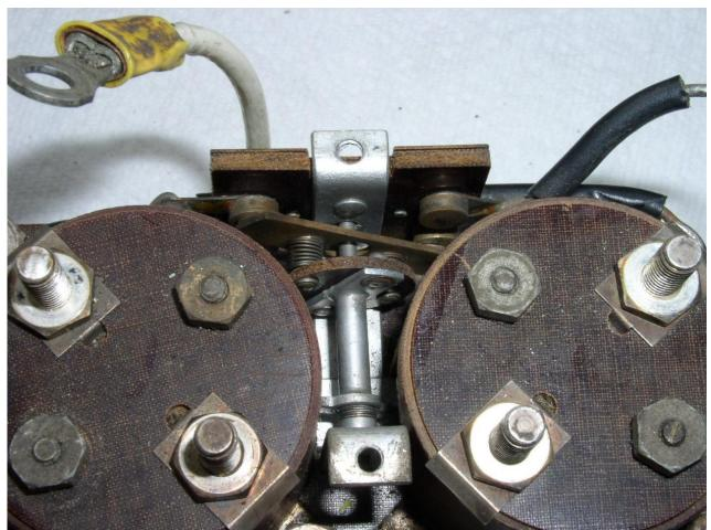
9. The shuttle switch contacts, shown above and at para. 5, are also subject to tarnish but aren't as readily removed. The contact plate is spring loaded so with the relay apart there is good access and it's easy to insert a fine point file or piece of Scotchbrite to clean up the contacts. While gently pinching the contacts together, slide a business card or similar heavy paper between the contacts for final cleaning.
