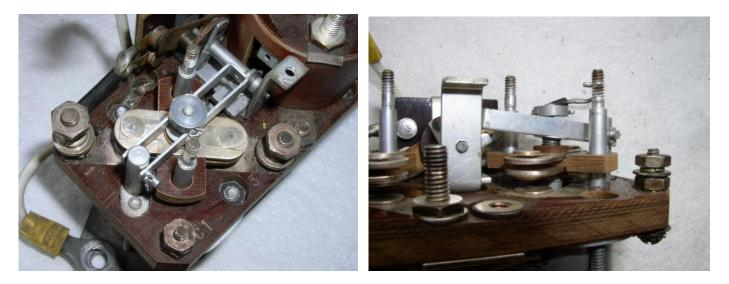
6. These photos show more clearly the upper relay contacts and the layout of the lever mechanism that moves the shuttle switch. The contacts exhibit some tarnish and pitting. Each lever is cushioned with a small spring so it only pulls down on the shuttle switch cam when its solenoid is activated. The cam pivot is seen at the hole through the vertical aluminum bracket in the upper right picture.
