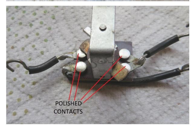
3. The lower fixed contacts shown earlier are easily removed for cleaning as shown below. The first photo shows the pitted contacts before removal. First take off the contact nut (top right photo), then loosen the attaching screw from beneath the base plate. The screw threads into the contact itself, shown lower left. The final photo shows the lower fixed contact after cleaning next to its mounting screw, and the mating movable lower contact plate to the left.
