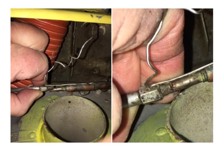
Another aggravating factor is the presence of sleeving or tape that is sometimes installed on the fitting shank for identification as an aid during initial airplane assembly. Corrosion can form more quickly underneath this material and be hidden from view during an inspection as shown in the following photograph. This material has no functional purpose on an assembled airplane.
