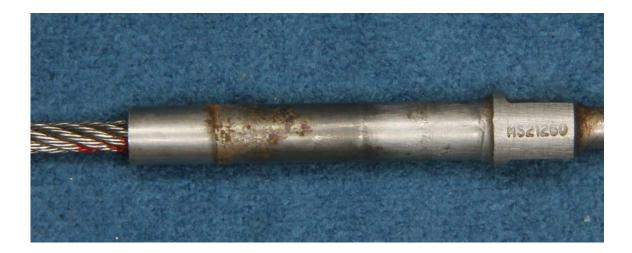
Again, because stress corrosion cracking is usually preceded by or accompanied with visible corrosion on the fitting, any corrosion visible in the area of the fitting is cause for concern.
