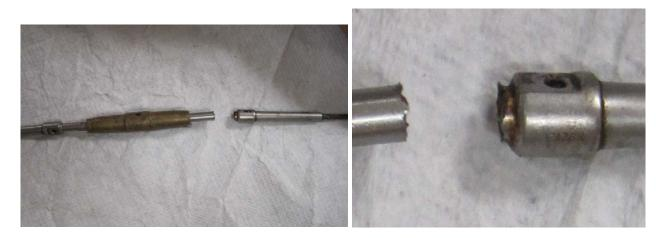
Depending on whether safety wire or a safety clip is used to secure the turnbuckle, any corrosion such as this may be hidden from view by the safety wire, which needs to be removed in order to perform an adequate inspection. The following photograph shows a typical safety wire configuration.
