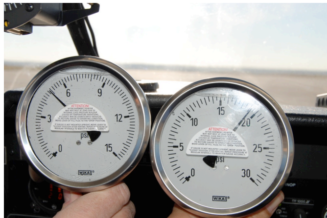
Photo 1: Standard pressure gauges - upper deck pressure of 4.9 PSI on left, metered fuel pressure of 19.2 PSI on right
