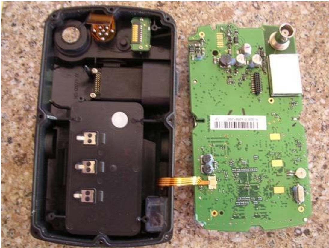
Here's the other side with our round coin battery. The stock battery is made in Germany and rated at 3VDC ~7mm diameter. It is soldered to the board with 2 tabs. The tabs are spot welded to the battery. Use a Volt Ohm meter to verify the +/- direction and write it down.
