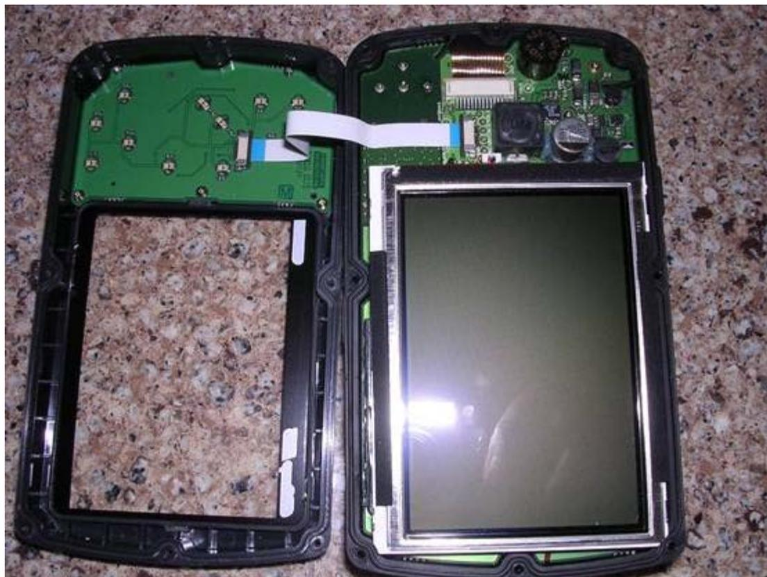
Remove the white ribbon cable that goes top both halves by gently sliding it out of the slot on the "screen" half.
