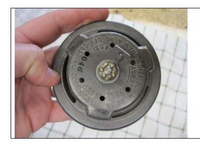
Tighten the nut until it feels pretty good to open and close the handle but do not put the cotter pin in yet. Go back to the plane and try the gas cap on. Fiddle with the nut until it is tight but not so tight that you need to pry the handle up with a crow bar. When it feels comfortable put the cotter pin in as show in the first picture.
