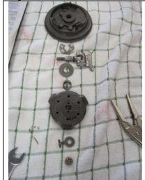
Take the handle and remove the small O-ring and install the new O-ring. Mike suggested some DC-4 to lubricate the shaft.
