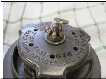
Make note that the eye of the cotter pin is vertical and note the position of the two legs of the cotter pin in this pre-disassembled picture. Use some pliers to remove the cotter pin and a wrench to remove the nut and you should see the following parts going from the top of the picture to the bottom: top of gas cap,  $\frac{3}{4}$  washer, handle, full washer, spring, bottom of gas cap, washer with tab for the chain, and nut with hole in it for the cotter pin.
