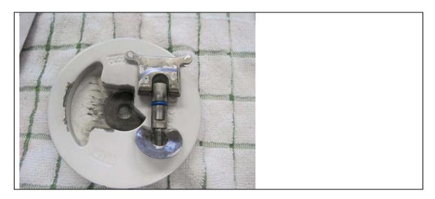
Now the next part is a little tricky because you have to push the handle (and ¾ washer) all the way down on the top, put the full washer on, put the spring on, put the bottom of the cap on while lining up the notch on the handle with the notch on the bottom cap, add the tab washer, and finally the nut. Here are some pictures to help.
