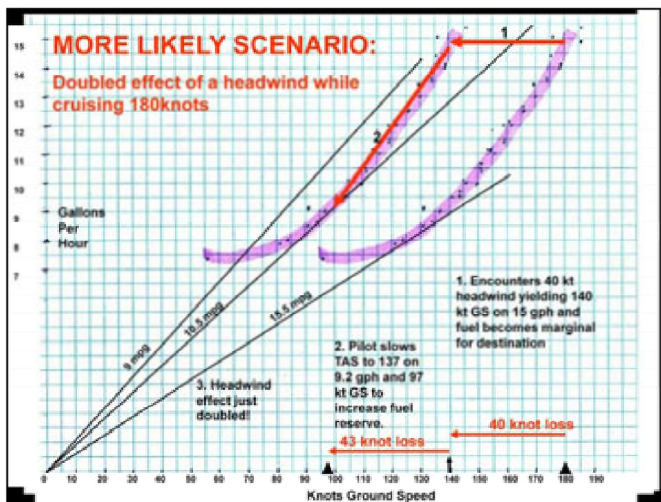
This is a more likely scenario showing that at normal cruise speeds, range is increased by slowing down in a headwind, in which case there is a doubled negative effect on ground speed.
