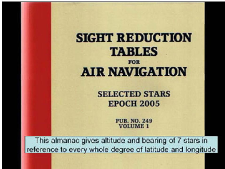
HO 249 offers altitude and bearing of 7 stars at every whole degree of latitude and longitude. The spherical trigonometry is all done by this almanac, and the remaining tasks are procedural and logical.
