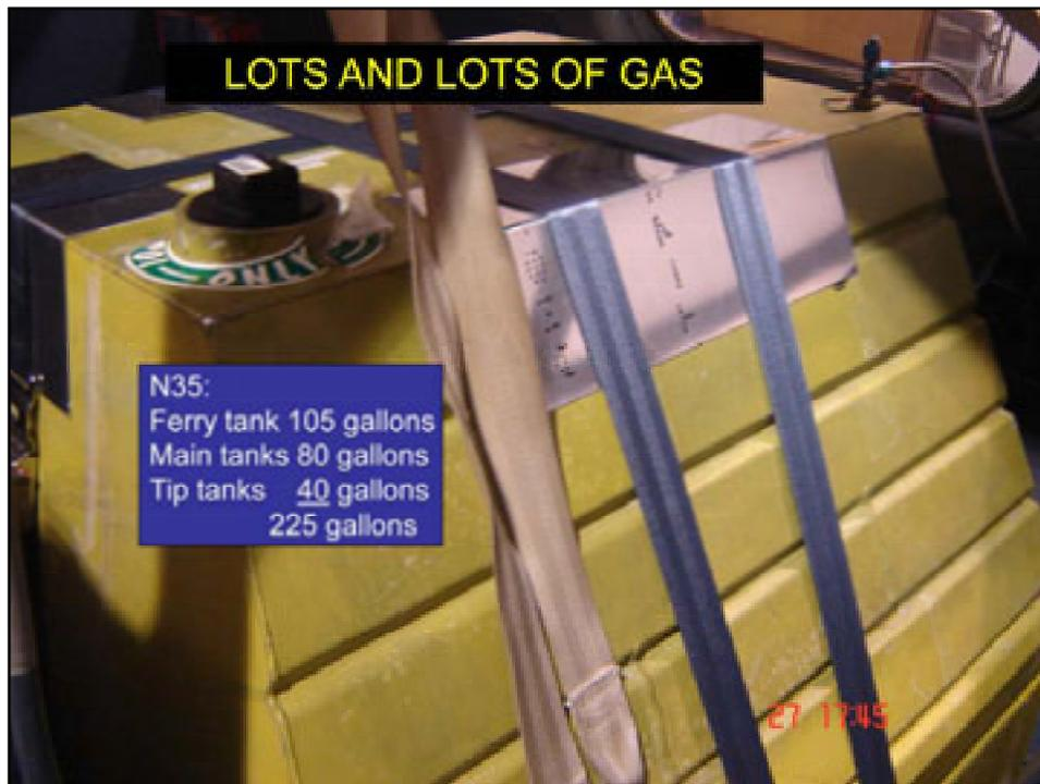
This is an aluminum ferry tank designed for Beech aircraft. There are now bladder tanks available which also will do the job.
