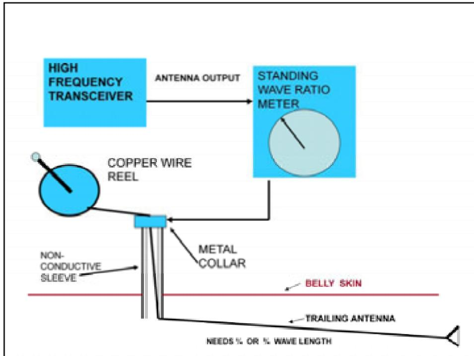
High frequency communications are needed for oceanic flight. HF radios have special antenna needs.
