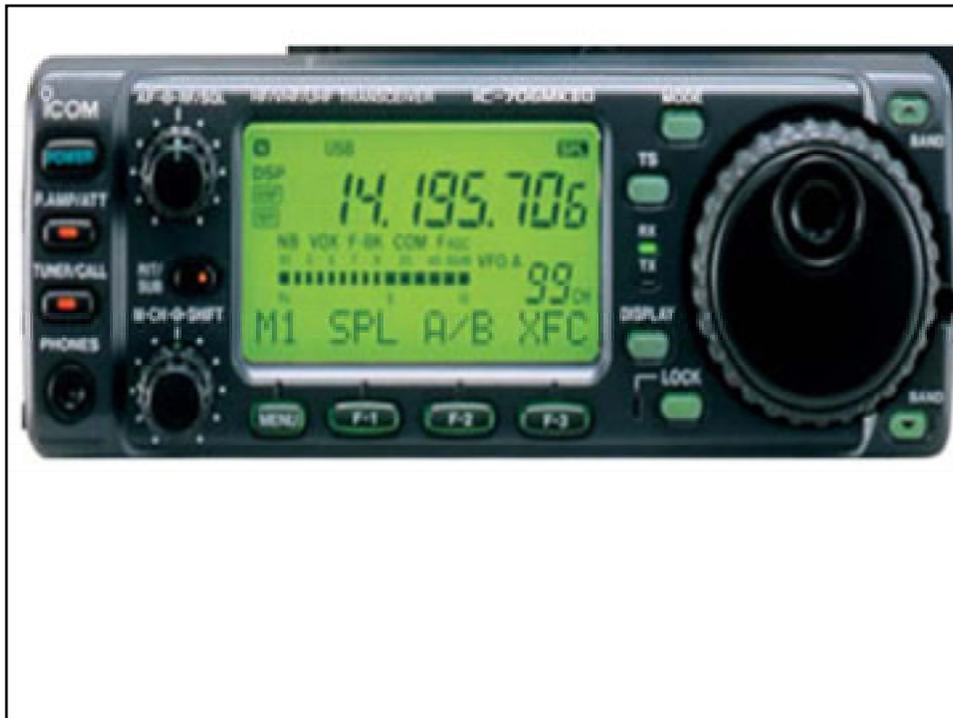
Here is an alternative to the trailing wire antenna. An antenna “tuner” or “coupler” can electronically tune a fixed length antenna to the correct wavelength. This Icom HF transceiver with AH-4 coupler requires 23 feet of antenna length, which means stringing the wire from roof to tail to wingtip on the Bonanza. The cross-ways antenna adds drag and collects ice easily.
