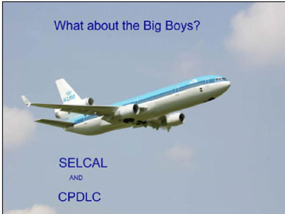
Listening to HF radio there is static which cannot be squelched out. Because of fatigue from listening, the airlines have a system called SELCAL. Each flight has a code, a series of aural tones which alert the flight crew to turn up the volume on the HF radio to receive a message.
