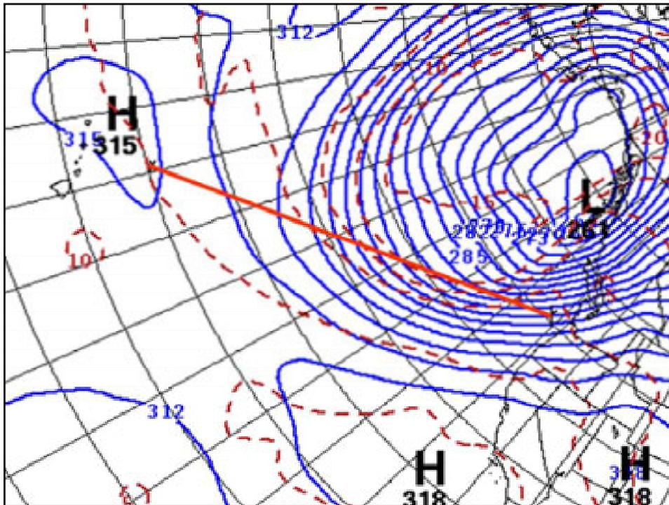
The flight plan ZIGIE to SEDAR intersections, using forecast winds, had wind correction angles of -11 degrees at halfway changing to +7 degrees approaching SEDAR.
