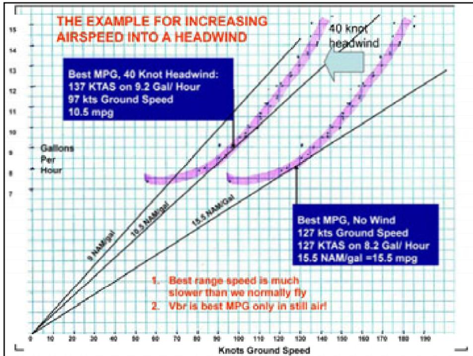
For the purple curve on the right, there is no wind, so airspeed equals groundspeed.
