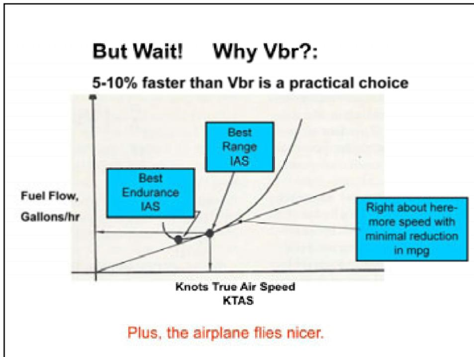
This is what the airlines did for oceanic cruise control with prop aircraft. The idea is that a 5-10% increase in speed over  $V_{br}$  causes minimal reduction in range, and makes a good trade-off.
