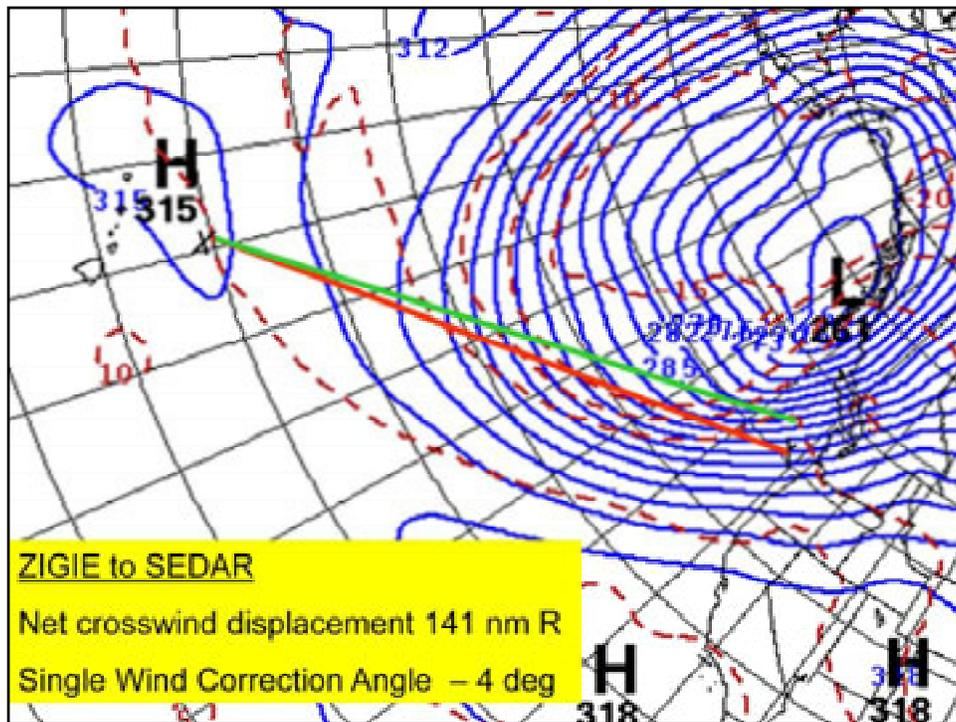
The Jeppesen CR3 computer takes true airspeed (155kts), mid latitude (35 deg), pressure drop (- 600 ft) and gives net crosswind displacement ZIGIE to SEDAR as - 141 nm.
