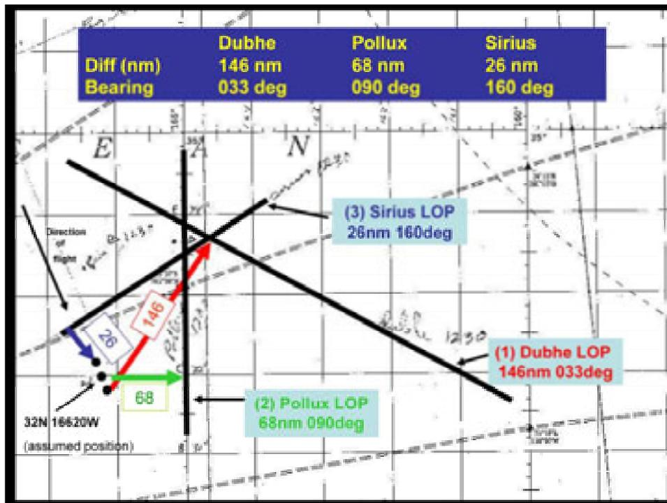
The difference and bearing of Dubhe was for a shot at 1226 hrs at the AP 32N16620W. But, our fix is for 1230, and in that 4 minutes the aircraft progressed 10 miles on a southeast course: therefore we plot the Dubhe LOP from a point 10 miles SE of the assumed position (“advancing the LOP”).
