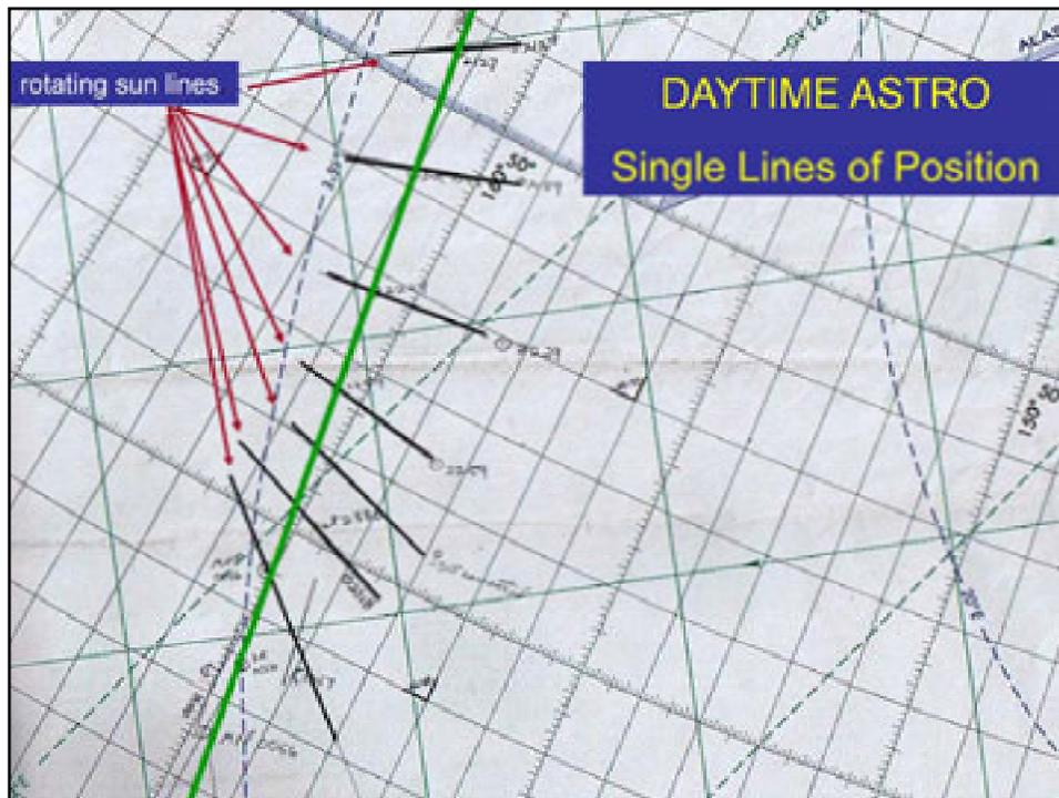
Daytime flight is less demanding than night flight, except the stars are gone. So for Astro, the navigator usually has only the sun for guidance. That's known as Single Line Of Position (SLOP) navigation. It is most useful around noon, when the angles change quickly- as in this slide.
