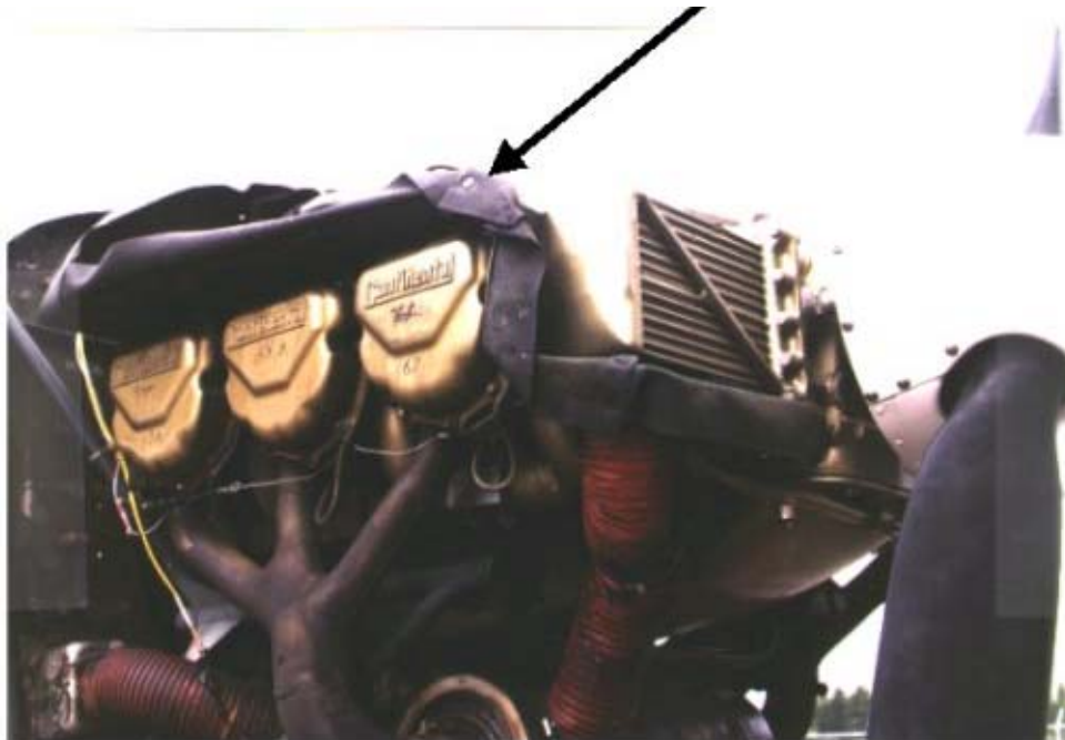
FIGURE 19-19. BAFFLE SEALS IMPROPERLY POSITIONED
