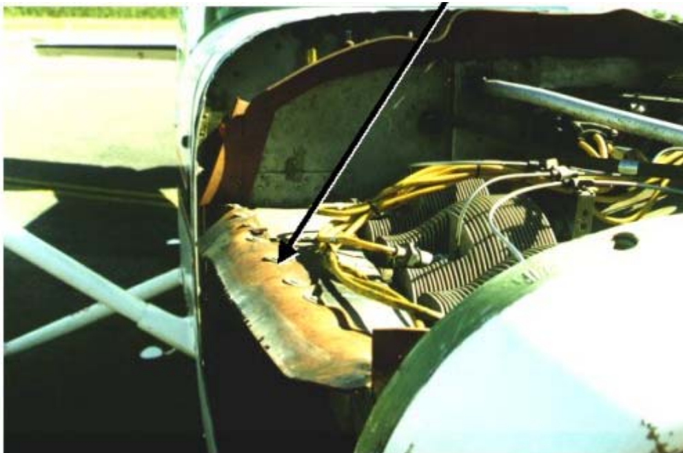
FIGURE 19-20. BAFFLE SEALS NOT SEALING PROPERLY
